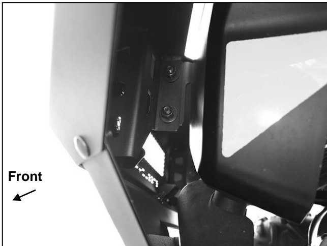
(Fig 12) Driver/left side of Bumper attached to Frame Bracket and Lower Skid Plate Mount Bracket
