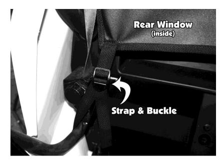
d. For now, leave the sides of the Rear Window unfastened. We will get to that after the Doors are installed. If you are not planning to install the doors at this point you can go ahead and attach the sides like you did the previous points along the top of the Rear Window.
