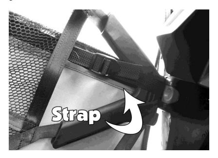
g. Now you can go back to the sides of the Rear Window Panel and run the straps on the Rear Window through the ladder lock buckles on the Door Panels. You will not need the double-sided Velcro strips sewn to the Rear Window and should tuck them away down between the two pieces. These Velcro strips are for when you want to install the Rear Window Panel without doors.
