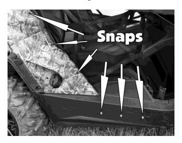
e. Save the two snaps on the front lower portion of the door until last. These will go into the plastic down around your feet and should be facing towards the rear of the vehicle. See Photo Below:
