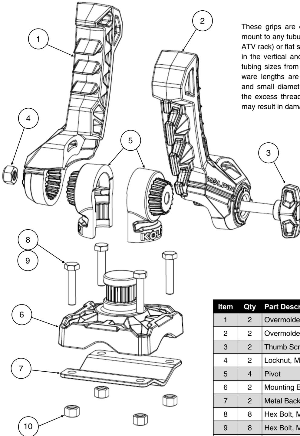
These grips are designed to quickly and easily mount to any tubular bar (example UTV roll cage or ATV rack) or flat surface. The grips can be mounted in the vertical and horizontal positions. The kit fits tubing sizes from 3/4" to 2.0" diameter. Two hardware lengths are provided to accommodate large and small diameter tubing. You may need to trim the excess thread once installed. Failure to do so may result in damage to your vehicle.
