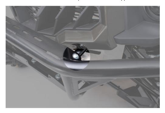
3. Using the provided **(2) M8-1.25x20 Allen Bolts and (2) 1/4" Flat Washers** loosely secure the headlight guards in the location of the previously removed hardware. Do not tighten.
