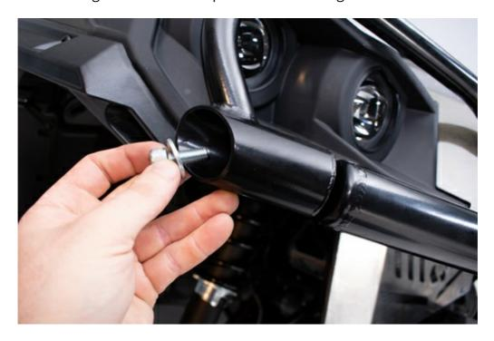
5. Tighten the smaller M8 allen bolts first then proceed to tighten the larger M10 allen bolts into the bumper end caps.
