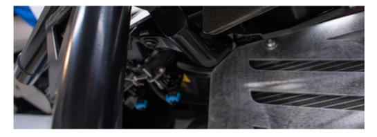
4. Use the provided **(2) M10-1.5x25 Allen Bolts and (2) 3/8" USS Washers** to secure the ends of the radiator guards to the bumper ends. Do not tighten.
