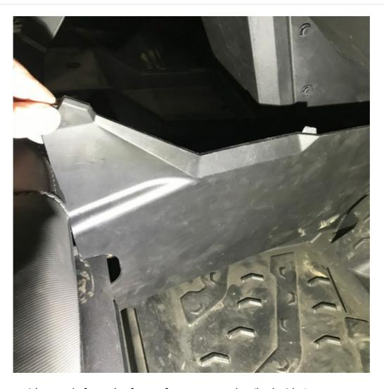
1. Remove side panels from the front of center console. (both sides)
