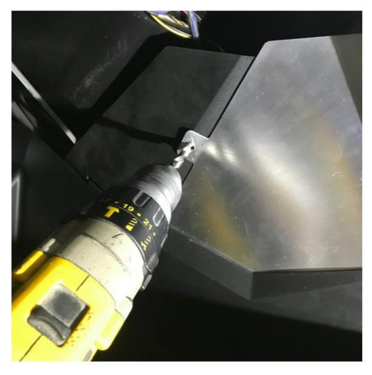
5. Making sure the new panel is sitting in the correct location drill second 3/8" hole through the plastic and install **punch pin**. (Both sides)
