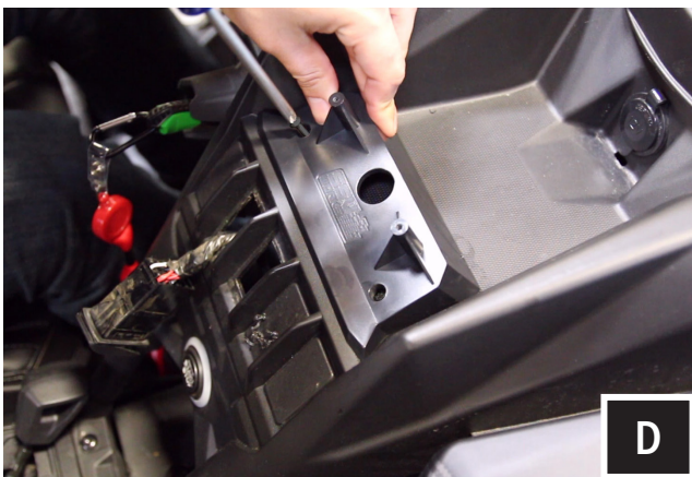
D. Place the base plate back on the dash lining up the outside screw holes to the dimples on the dash. Using (2) #7 Screws and a philips screw driver secure the base to the dash. Make sure the screws are driving into the dash dimples for best results.
